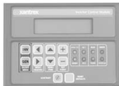
Figure 5-3 ICM ON/OFF Push-buttons
