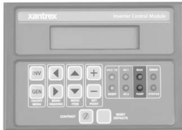
Figure 8-4 Charge Status LEDs
