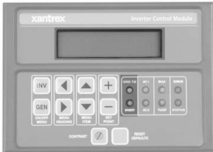
Figure 8-2 Inverter Operation Status LEDs
